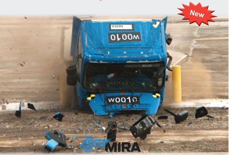
photo shows result of test at 48 km/h
